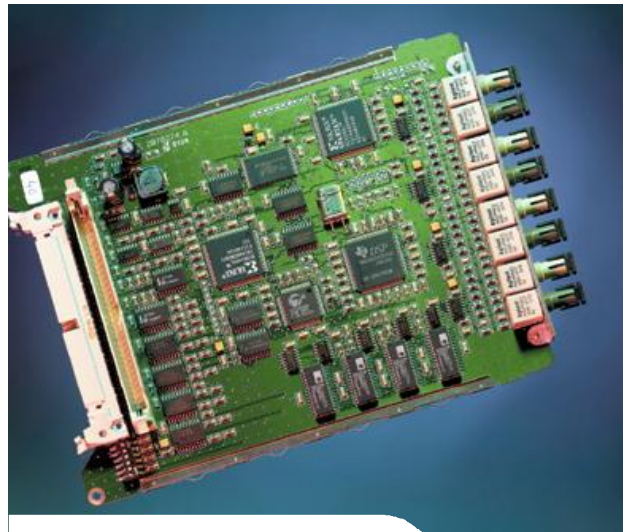
Figure 7.8: Circuit board for numerical relay
