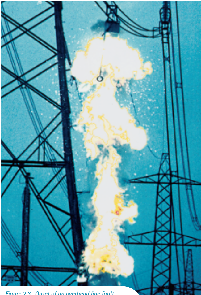
Figure 2.3: Onset of an overhead line fault
